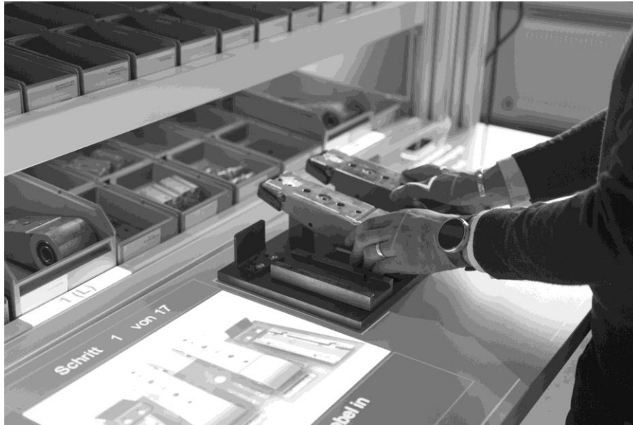
Figure 3: Projection-based assembly assistance system.
